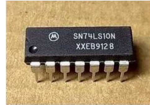
74LS10 3x 3-input NAND Gate (in somewhat obsolete DIP-14 package)
